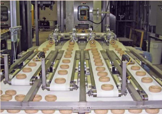
++ After leaving the kneader, the dough passes through the divider to obtain dough pieces, which are then shaped and rolled around a shaft to give the bagels their characteristic ring shape
