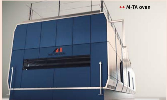
The bagels move on to the oven where they will be traditionally baked on the floor or hearth of the oven. Depending on market expectations, the hearth of the oven is available with or without marks. For a bagel with a smooth underside, FTP technology with metal bands is recommended; and for hearth marking, the M-TA oven technology is used.
