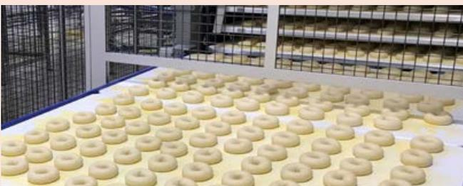
++ Placed on fermentation trays called peel boards the dough pieces enter the fermentation stage. Bagels generally require two-phase fermentation: parboiling at very high temperatures, followed by "retarding" in a cold atmosphere, to stop fermentation and to firm up the product by creating a thin superficial skin
