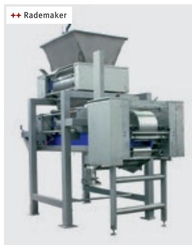
which achieves a dough reduction ratio of 8:1 without tension on the sides of the dough sheet.
