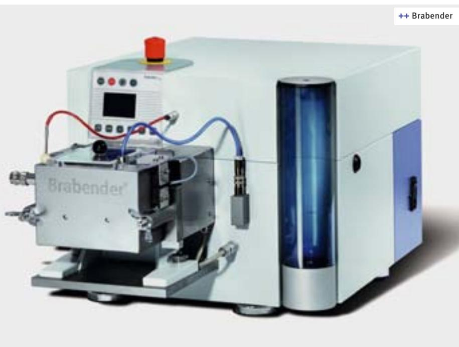
absorption and the rheological properties of dough and batters and for that, a flour-water suspension is filled into a heated measuring mixer. Rotating mixing tools subject the suspension to a defined amount of mechanical stress. The resistance of the dough is measured as a moment of force and plotted in a Farinogram. It shows the water absorption, dough development time, dough stability and degree of dough softening.
