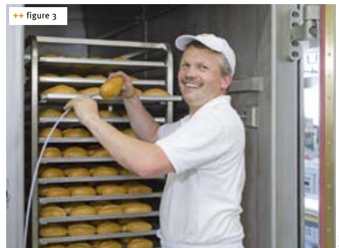
++ figure 3 A measuring needle reports values from the interior of the roll
