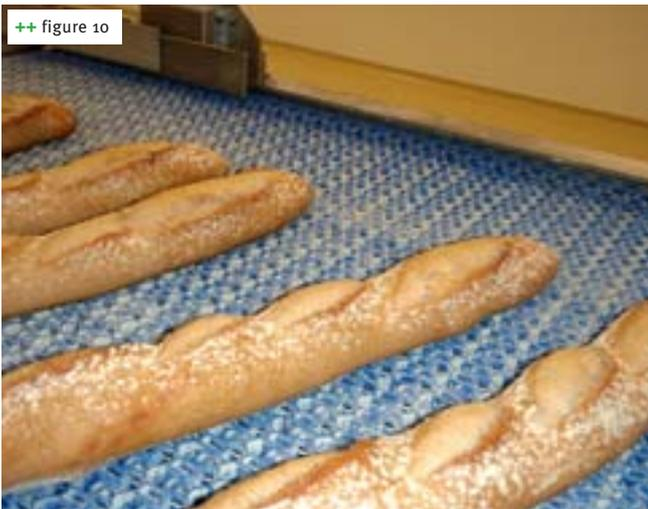
pieces move back and forth through the pre-proofer. At each end they are turned and placed on a belt underneath. In this way, the side that has just dried comes into contact with the belt and sticking to the belt material or smearing is prevented as a result.
