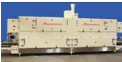
Macrowave™ Post-Baking Dryers utilize RF (radio frequency) energy which preferentially heats and dries the moist areas of cookies, crackers and snack foods to eliminate surface checking and control moisture and color. Capable of increasing productivity by 30% or more, these dryers remove the drying requirement from ovens to let bakers maintain their oven settings to achieve the product color goals in the last third of an oven line.
