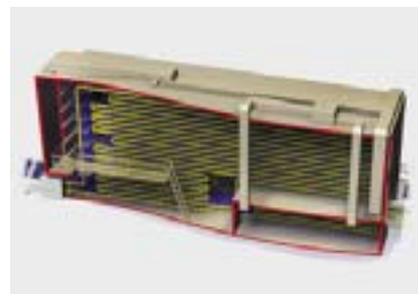
The hallmark of Auto-Bake's Serpentine technology is the S-shaped transport path, where trays are conveyed over multiple levels without tipping. The Serpentine proofing system utilizes Auto-Bake's increasingly popular 'free tray' system, where the trays are independent of the oven, allowing makeup and forming to take place on existing equipment. According to Graeme Bonner, Auto-Bake technical sales engineer, the automated Serpentine proofing process conveys a number of advantages.
