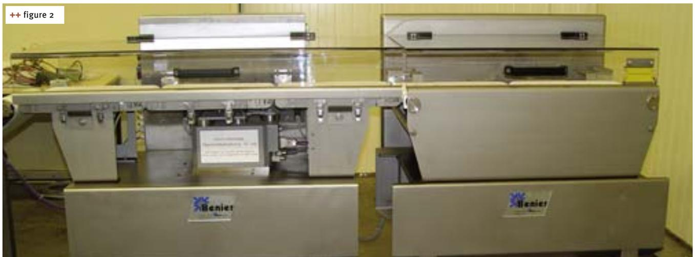
charged from the divider. Based on the distribution of weights, the optimum suction volume is calculated for the dough just being processed and the Dough Master controlled accordingly. The end result is a narrower curve of distribution, higher weight preciseness and less stress on the dough.
