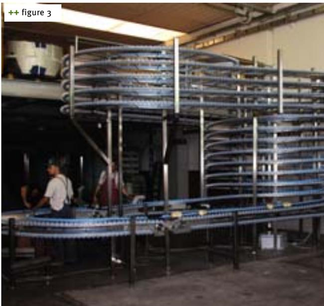
clearly lower than in former plants. In addition to that, the drives will be located on the outside making them easily accessible. They can move the belts forward and back, so that the spiral towers can also be used as buffers for the production lines if needed.
