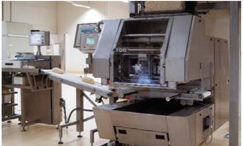
Firstly, all knives, pistons and peels are driven independently via servo motors and are computer-controlled, based on the respective recipe. This has the advantage that the movements during dough division are not parallel and that the dough is only pushed into the weighing compartment when the suction piston has really reached its ultimate position. In addition, the pressure of the suction piston can also be controlled depending on the recipe.
