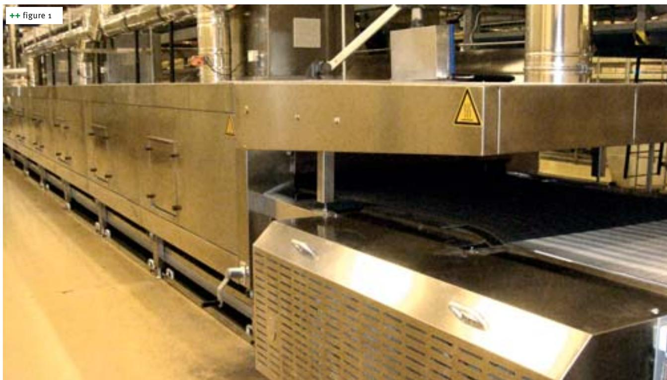
**+** The outstanding feature of the hybrid oven is the first zone where the products are baked in the first half with radiation heat followed by convection heat in the second half and all other following sections. In this way, DFE Meincke triggers a strong initial baking process ensuring proper oven spring – a process formerly performed by pre-baking ovens.
