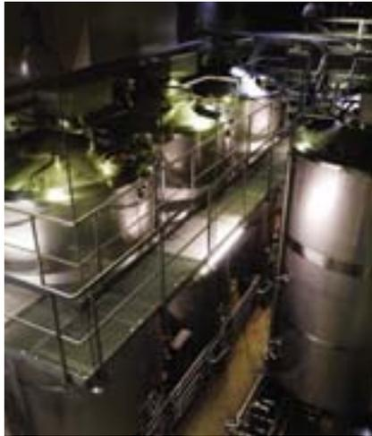
++ New fermentation tanks for the production of sourdough
