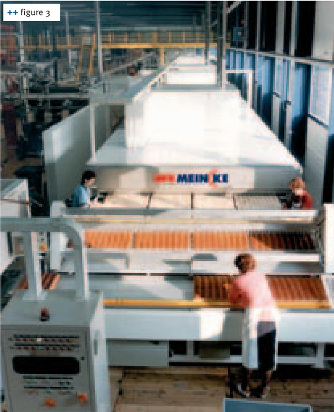
independent control for heat, humidity and air circulation. The inside of the oven is made from Cor-Ten steel, which is very resistant to humidity, or from stainless steel. All ovens are set-up and tested prior to dispatch.
