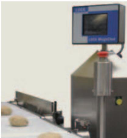
Installed after the dough rounder, by which stage the dough is less sticky, a fixed table dough weighing unit was incorporated in the line with two in-feeds to create the appropriate pitch. A reliable reject mechanism was a vital component as a faulty device can bring the whole line to a standstill. Crucially, the "lift and drop flap" reject supplied by Lock means under- or over-weight
