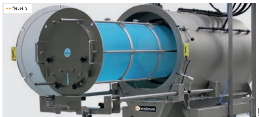
++ figure 3 A fast opening system for sifters
