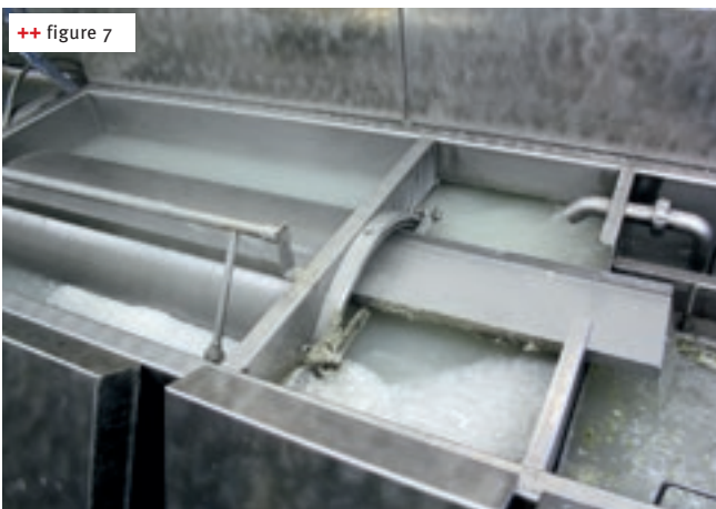
++ figure 7 The washing liquor is purified via the drum filter from the inside to the outside installed at the side. The dirt remains on the inside of the drum wall
