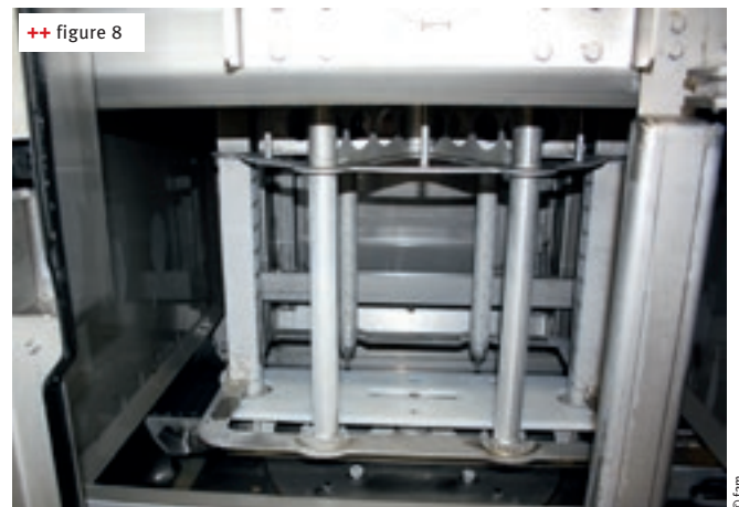
++ figure 8 In the drying centrifuge the stacks of 10 baskets land on the white turntable, where they are held in position by the descending basket before being spun for approx. 5 sec
