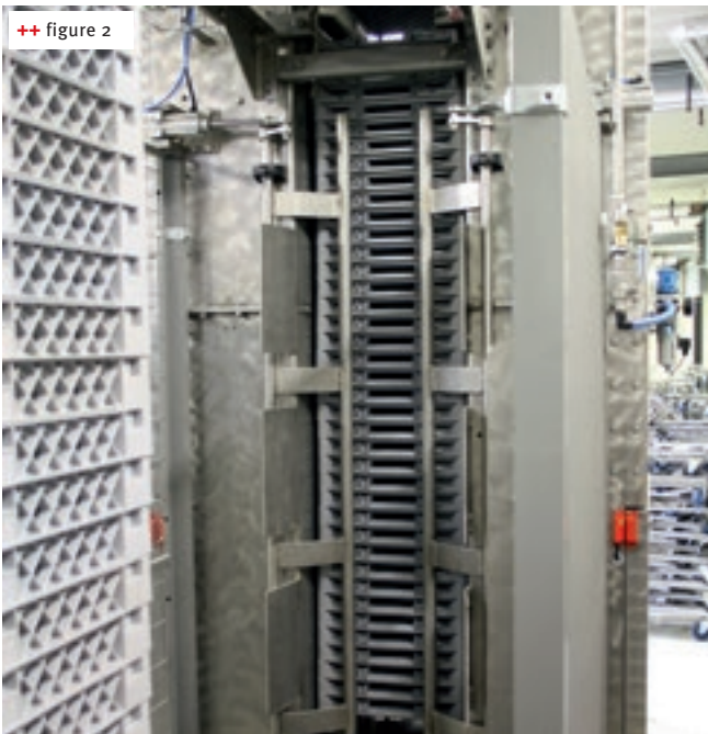
++ figure 2 In the destacker the baskets are fed into a kind of turnstile in which the baskets are removed from the stack individually, starting at the top
