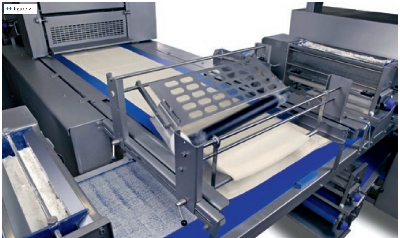
++ figure 2 A cut & stack laminating section
