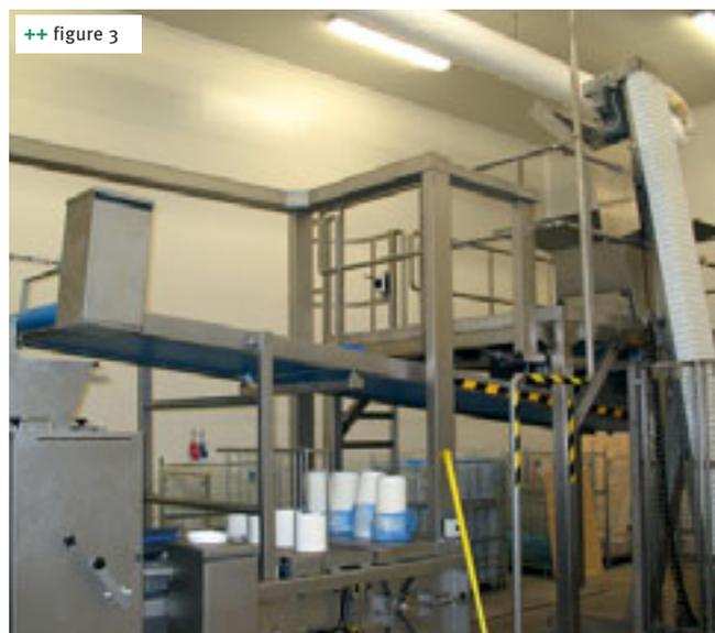
line from Rademaker. This PLC controlled line, made of stainless steel and completely wash down, produces 4,800 quiches per hour. The demand for quiches is increasing not only from within the Netherlands, but from Germany, Ireland and France as well. The expectation is that within three years, the commissioning of a second line will be needed.
