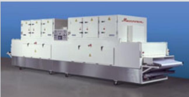
A series of post-baking dryers that can be custom engineered for cookie, cracker, and snack food production operations in order to increase oven band speed by eliminating the final drying requirement from the last third of an oven line is available from Radio Frequency Co., Inc. of Millis, Massachusetts, USA.
