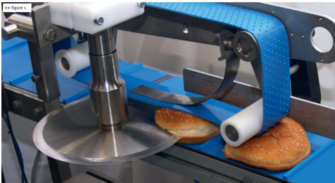
+ Impressive equipment, presented at the stand of Döinghaus Maschinenbau GmbH during Anuga Foodtec, stirred up the interest of the representatives from the baking industry. Underneath a swivable cupola, Döinghaus, long term suppliers of cutting machines for the baking industry and Herrmann Ultraschalltechnik, demonstrated a new development: an ultrasonic circular knife that can be used horizontally and vertically. The knife is only 2 mm
