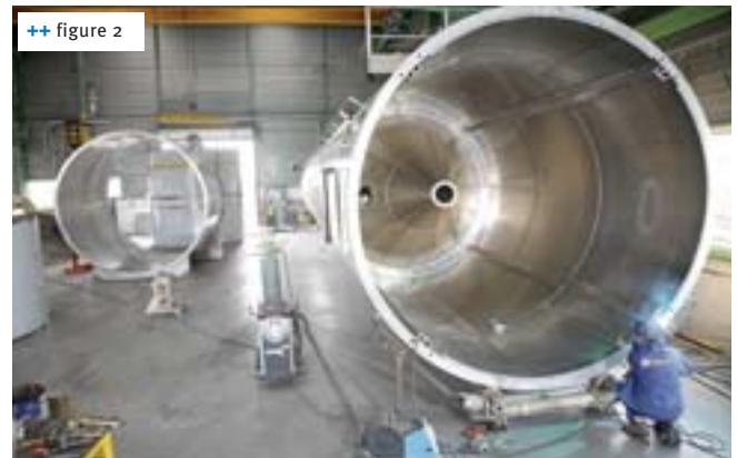
++ figure 2 Manufacturing of aluminum silos
