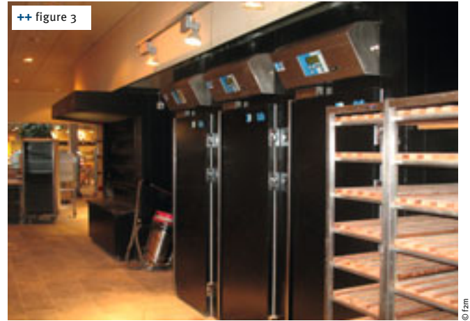
++ figure 3 The multi-deck oven in the background bakes the whole bread range, part of which is stored in PATT cells (front)
