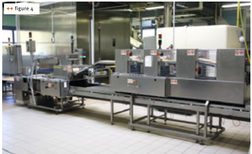
++ figure 4 Processing sticks such as grissini, beer sticks and salty pretzel sticks on modern plants; 12-15 t of baked goods leave the entire production unit every day
