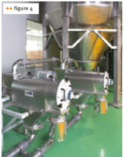
foreign particles when products are being charged. Vibrating screens assist the flow of non-free-flowing bulk solids. Vibrating grits with breaking device break up clumps carefully. Vibrating screens are also available with automatic segregation of foreign particles (see figure 3).
