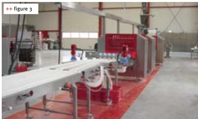
**+** The modular designed laminating plant is intended for large craft and industrial bakeries which are able to invest into a machine with an hourly capacity of up to 5 tons of dough.
