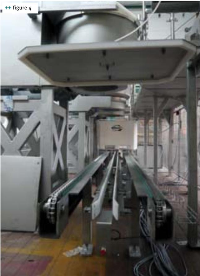
ports it to the bowl lifter from where the dough is moved to the dough make-up station. The main advantage of such a system is the parallel production of different products – in this case pizza, bagels, bread and rolls – which require different dough resting times. Before the dough resting vats are moved underneath the mixers, a fine oil film is applied on the inside of the vats at an upstream station. This prevents the dough from sticking to the walls of the vat.
