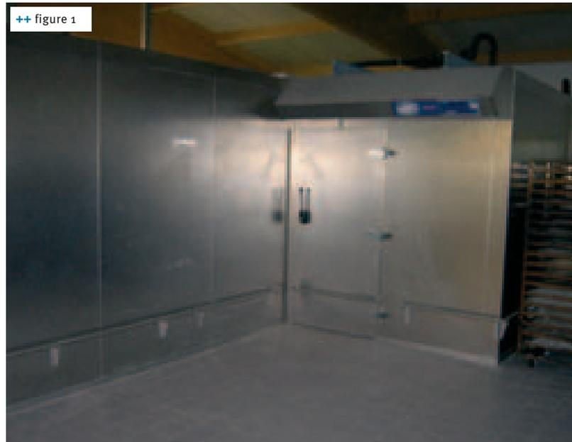
in the new shock freezer was very even from the beginning which can not be said of the older system (not made by Hein) that had posed problems for many years. The storage temperature in the new frozen storage is absolutely uniform without any loss of volume or drying out of the dough pieces as had happened with the older plant. Most of the dough pieces are stored unpacked. Even after one week in storage there is no noticeable difference after conditioning and baking."
