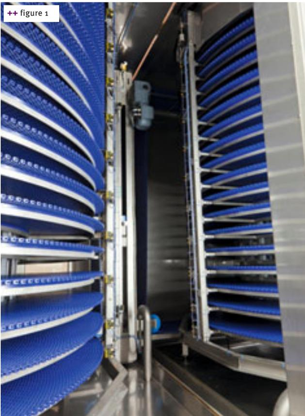
++ figure 1: The compact duo. – a double drum system with 2 x 18 tiers
