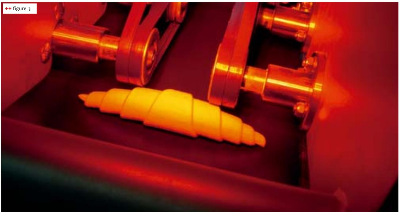
system (seam position control system), Fritsch guarantees a position preciseness of  $\pm 15$  degree. The processing speed is about 70 cycles/minute. The line speed is only limited by the performance of the camera software. Efforts towards further increase in performance are already in the pipeline. With this equipment, the detection is much more precise than with other systems and, according to the company, the error rate is less than 5%.
