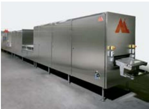
One version of the new Jensen Line is for making solid moulded chocolate tablets with or without inclusions such as nuts or rice crisps. The output for this line is up to 800 kg/hr and the speed is 15 moulds/minute. The depositor can also be used for making one-shot products. A wide range of additional tools are available for the production of filled products, products with biscuits and wafers, cold-pressed
