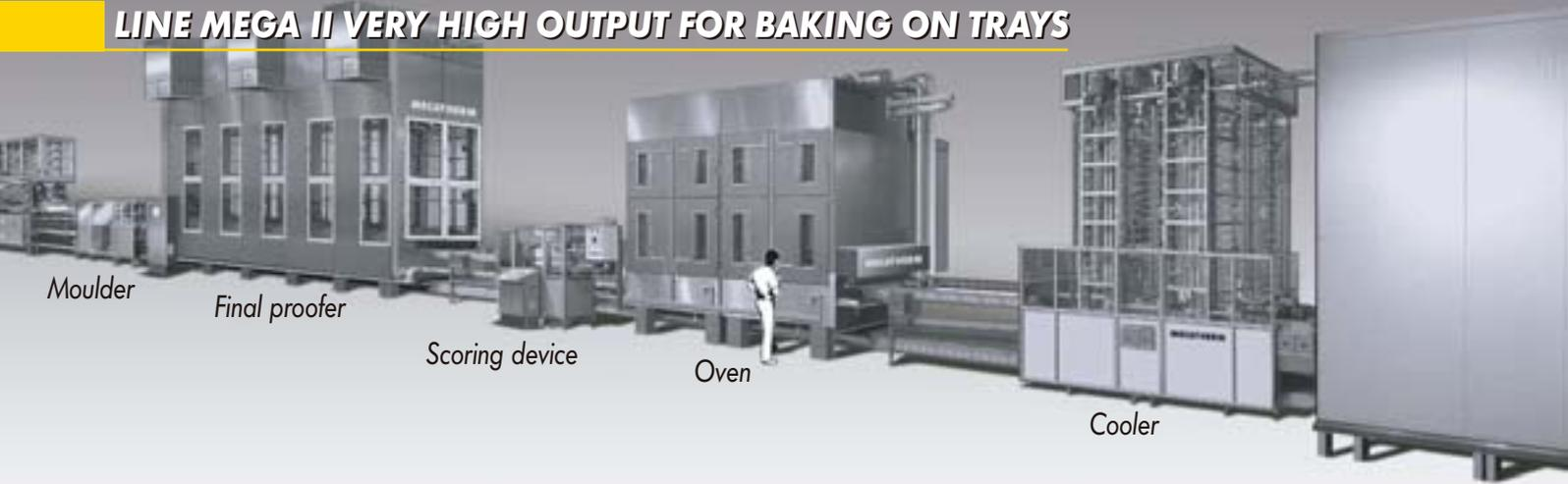
**MECATHERM** produces fully automatic lines as well as individual equipment such as moulders, ovens, spiral coolers and freezers...
