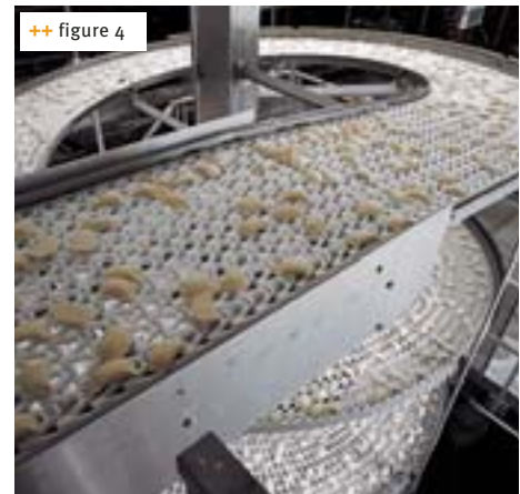
++ figure 4 ProLink Wendel from the modular belt range, produced in Denmark
