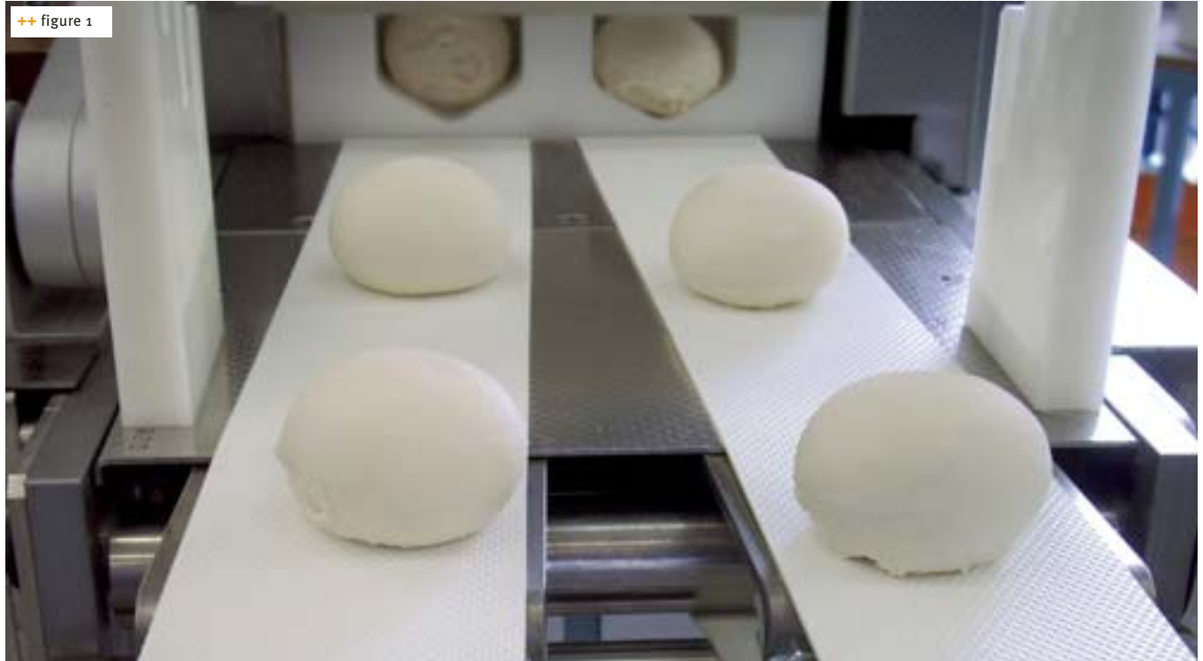
++ figure 1 New spreading belt with inverted pyramids surface
