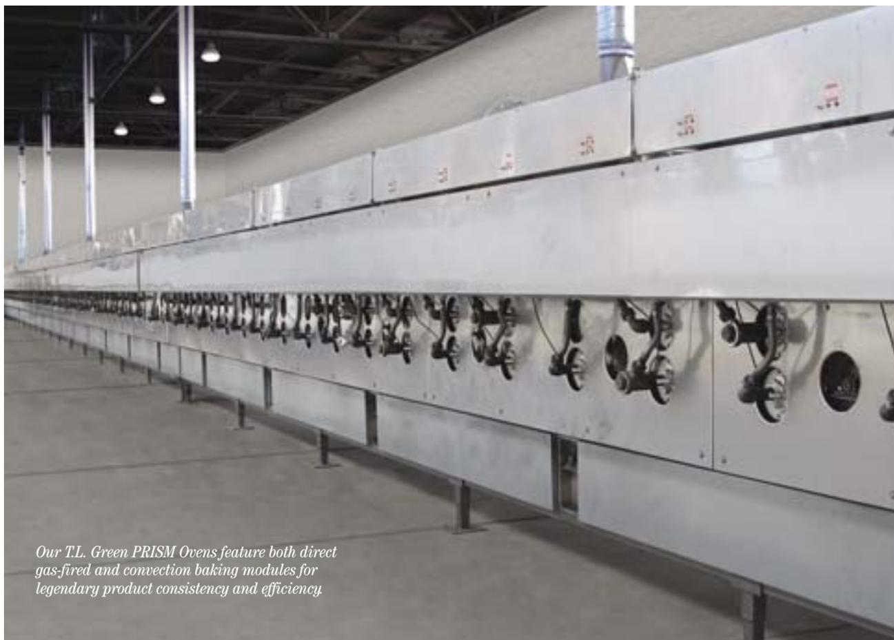
*Our T.L. Green PRISM Ovens feature both direct gas-fired and convection baking modules for legendary product consistency and efficiency.*
