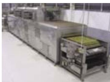
*Our double-pass SPECTRUM OVEN® with its variable heat flux, is truly a flexible platform for a wide range of baked snack products.*
