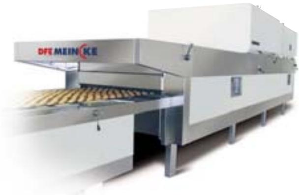
**Direct Three - Directly gas fired oven**
