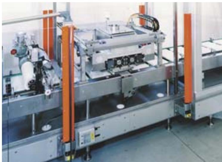
dients, with programmable pouring by means of the operator interface and PLC. The chocolate depositor is equipped with an electronic control system with the operator interface
