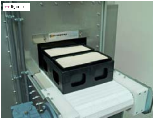
++ figure 1 The products are baked in special strap pans made from plastic material
