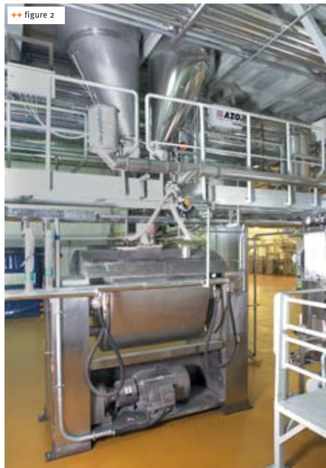
++ figure 2 Flour scale asymmetrical (left), sugar scale and kneader (right)
