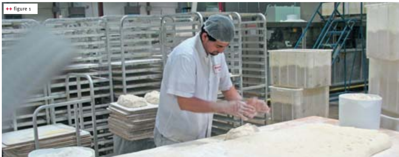
++ figure 1 Large “freeforms” called ciabattas are scaled manually and placed on peel boards
