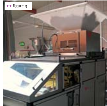
++ figure 3 Dough divider with transparent dough funnel
