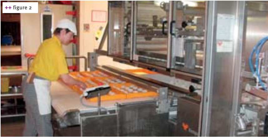
++ figure 1 Evolution – The new modular roll line by Kemper
